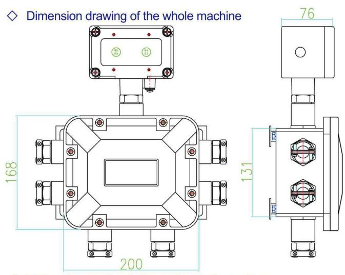
Main unit mounting holes and inlet dimensions
