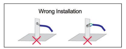
The ground wire is connected to the grounding stake with M8 bolts, and the two copper noses are connected separately.
